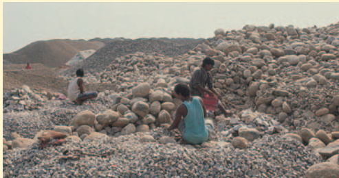
Labour based methods can effectively be used in producing aggregate for use in Otta Seals. (Bangladesh).
