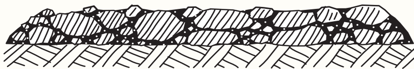
Single Otta Seal (0-16 mm). Thickness: minimum 16 mm
