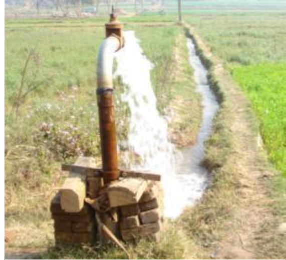
Figure 9-1: Typical Shallow Tubewell
